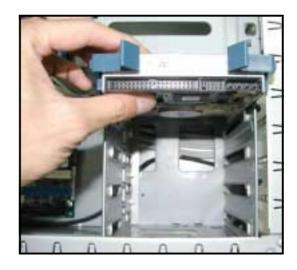
Connect the IDE and power cables to their corresponding connectors on the back of the drive.
